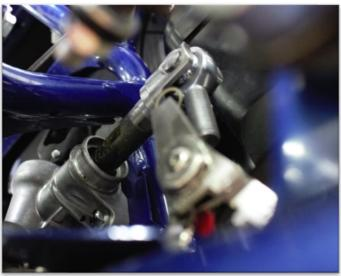
**Step 8:** The factory boot/bellow can be reinstalled. Slide the boot/bellow over the current assembly. Then fasten the RH 5/8" jam nut on the rod end.
