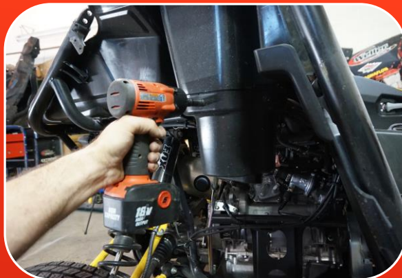
Remove the lower oil tank shroud using a 10mm socket
