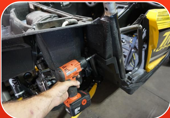
Remove the bed front inner bolts using a 10mm socket
