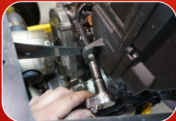
Remove the rear airbox mount using a 10mm socket
