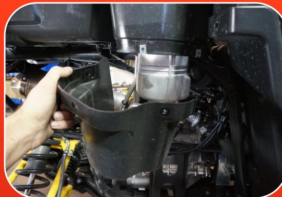
Remove the oil tank shroud
